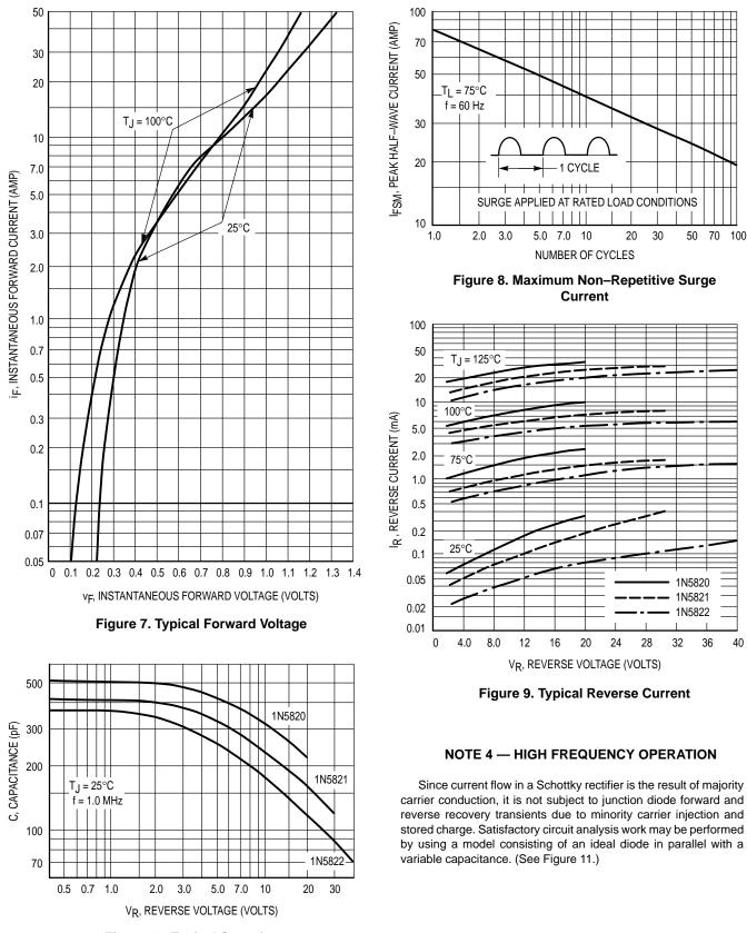
Figure 10. Typical Capacitance
