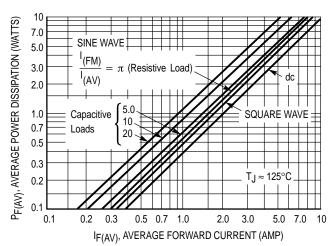
Figure 6. Forward Power Dissipation 1N5820–22
