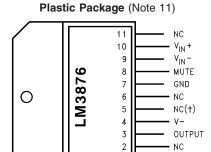
†Connect Pin 5 to  $V^+$  for Compatibility with LM3886.
