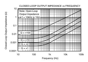
At  $T_A = +25$ °C,  $V_S = \pm 15$ V,  $R_L = 2k\Omega$ , unless otherwise noted.
