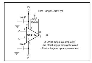
FIGURE 1. OPA134 Offset Voltage Trim Circuit.
