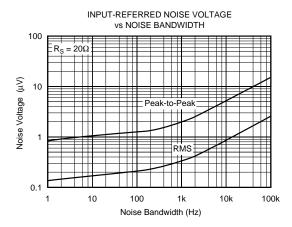
At  $T_A$  = +25°C,  $V_S$  = ±15V,  $R_L$  = 2k $\Omega$ , unless otherwise noted.
