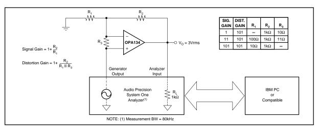
FIGURE 2. Distortion Test Circuit.
