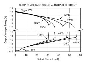
At  $T_A$  = +25°C,  $V_S$  = ±15V,  $R_L$  = 2k $\Omega$ , unless otherwise noted.
