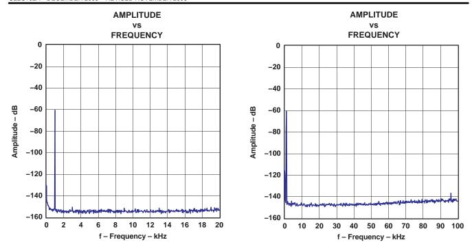
NOTE:  $f_S = 48$  kHz, 32768 point 8 average,  $T_A = 25^{\circ}C$ ,  $V_{DD} = 3.3$  V, NOTE:  $f_S = 96$  kHz, 32768 point 8 average,  $T_A = 25^{\circ}C$ ,  $V_{DD} = 3.3$  V,  $V_{CC} = 5$  V, measurement circuit is Figure 24.
