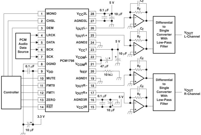
Figure 23. Typical Application Circuit
