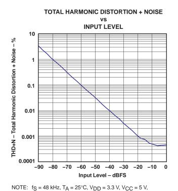
Figure 17. THD+N vs Input Level, PCM Mode
