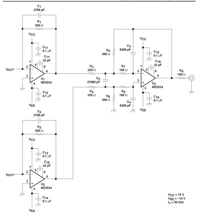
Figure 24. Measurement Circuit
