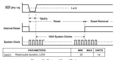
Figure 20. External Reset Timing
