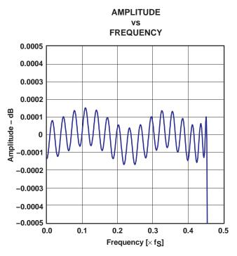
Figure 2. Pass-Band Ripple, Sharp Rolloff
