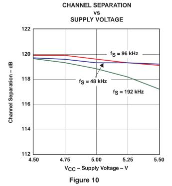
NOTE: PCM mode,  $T_A = 25^{\circ}C$ ,  $V_{DD} = 3.3$  V, measurement circuit is Figure 24.
