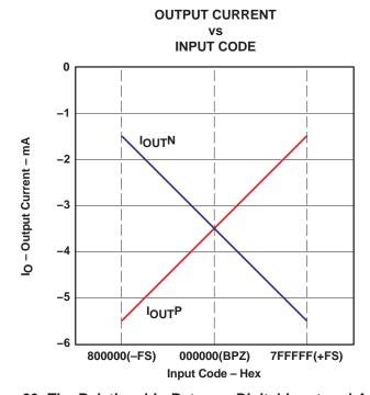
Figure 29. The Relationship Between Digital Input and Analog Output
