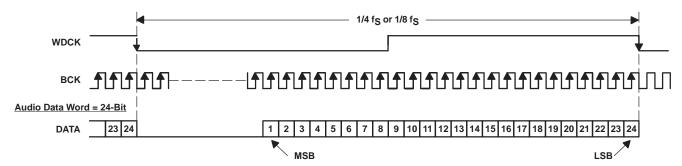
Figure 27. Audio Data Input Format for External Digital Filter (Internal DF Bypass Mode) Application
