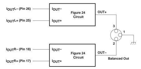
Figure 25. Measurement Circuit for Monaural Mode
