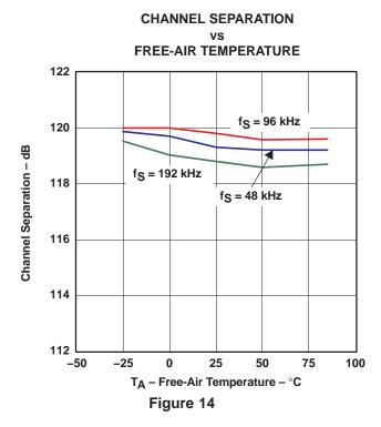
NOTE: PCM mode, V<sub>DD</sub> = 3.3 V, V<sub>CC</sub> = 5 V, measurement circuit is Figure 24.
