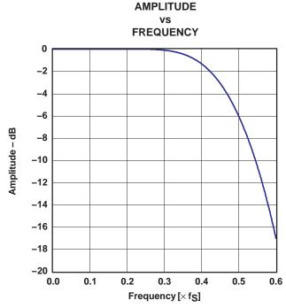
Figure 4. Transition Characteristics, Slow Rolloff
