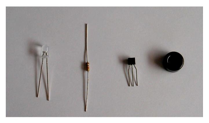
You're going to need a white or blue LED that is rated for 3 volts, a 1K resistor, a 2N 3904 NPN transistor, a toroid, two pieces of wire and a battery.
