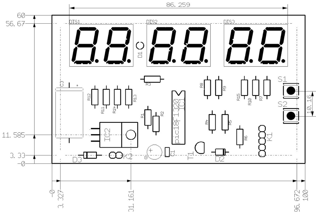
When mounting components – note that as there is no through plating, many component leads will require soldering on both sides of the board.
